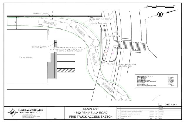
Supported by Staff, the applicant is proposing to close the northern single lane access and create a routing that goes through the existing drugstore parking lot to the rear of the property. The following sketch shows the proposed truck movements through the site (**Figure 3**).
